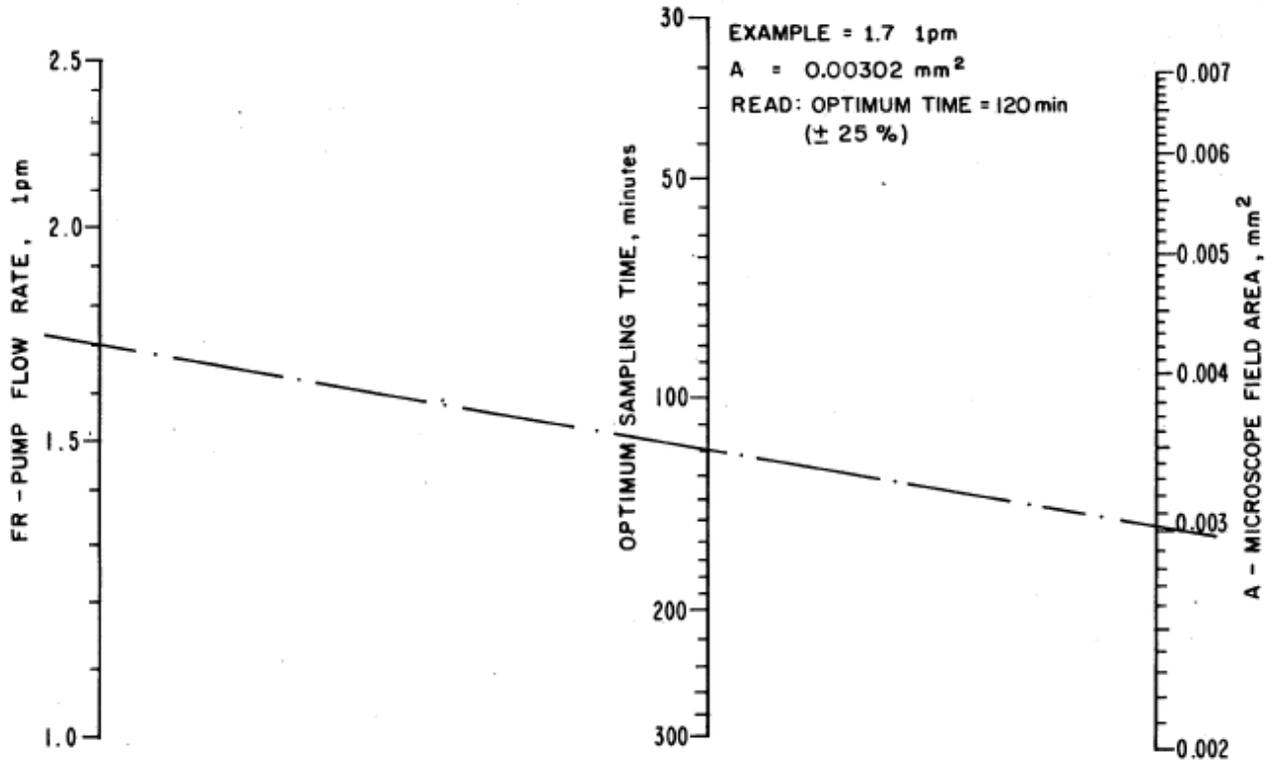
Figure 4 Nomogram of optimum sampling times for airborne asbestos fibers in concentrations of 1 to 10 fibers/cm<sup>3</sup>
