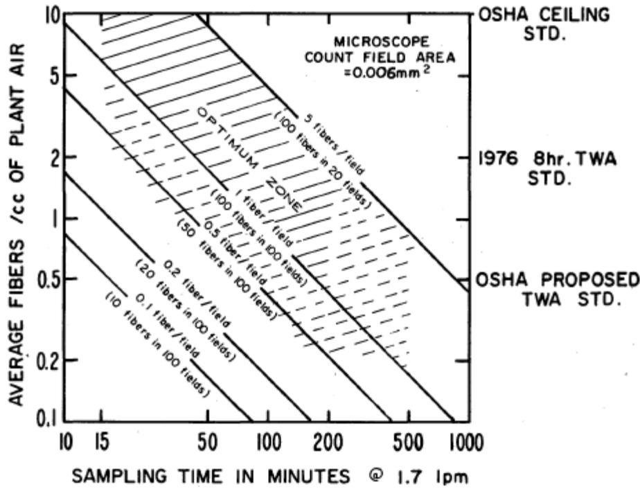
Figure 2 Optimum sampling times for airborne asbestos where microscopic field area = 0.006 mm<sup>2</sup>
