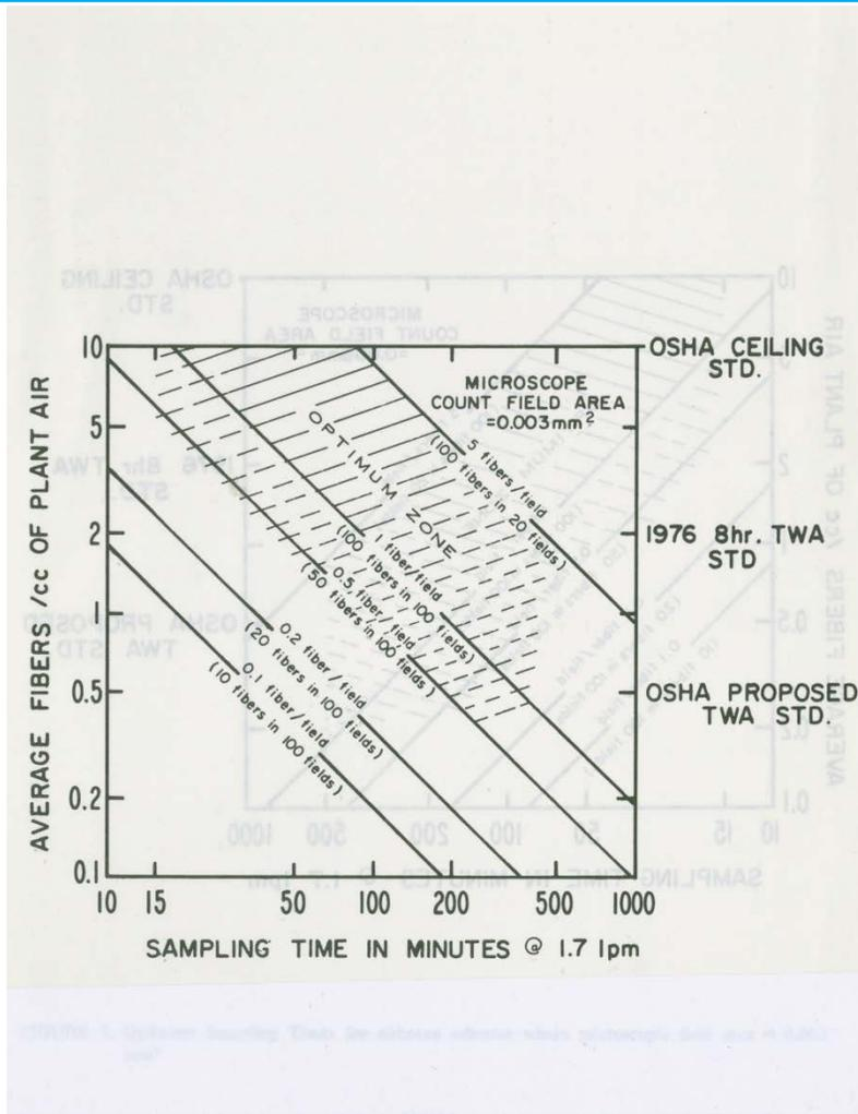
Figure 1 Optimum Sampling Times for airborne asbestos where microscopic field area = 0.003 mm<sup>2</sup>
